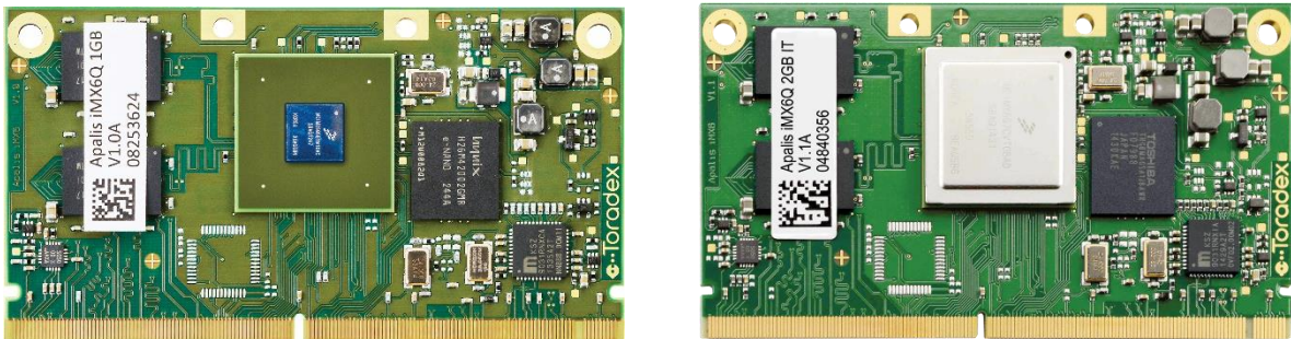
Figure 18 left side: commercial temperature module without lid; right side: industrial temperature module with lid
