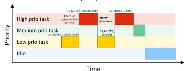
With priority inheritance, the low priority task inherits the priority of the waiting high priority task as long as it holds the mutex. The lower priority task is activated instead of the medium priority task when the high priority task tries to claim the semaphore.
