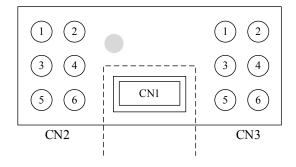
Pinout of the FPC5924 breakout board.
