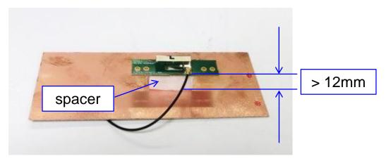
\*Recommended minimum spacing when the 1000418 antenna is installed over a ground plane
