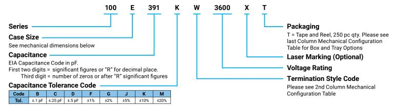
The above part number refers to a 100 E Series (case size E) 390 pF capacitor, K tolerance (±10%), 3600 WVDC, with W termination (Tin / Lead, Solder Plated over Nickel Barrier), laser marking and Tape and Reel packaging.
