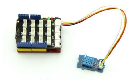
The Temperature and Humidity sensor is connecting to analog port A0 of Grove - Base Shield.
