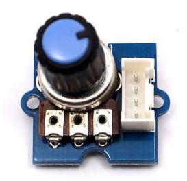
There is another production - Grove - Rotary Angle Sensor(P). What does "P" mean? "P" is for "panel mount" in this product. It is the sister version of Grove - Rotary Angle Sensor. They are identical except the Grove connecter is moved to the back so that you can easily use it as a neat and wire-free human interface device.
