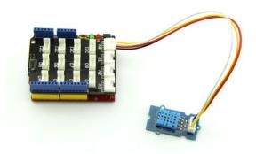
The Temperature and Humidity sensor is connecting to analog port I2C of Grove - Base Shield.
