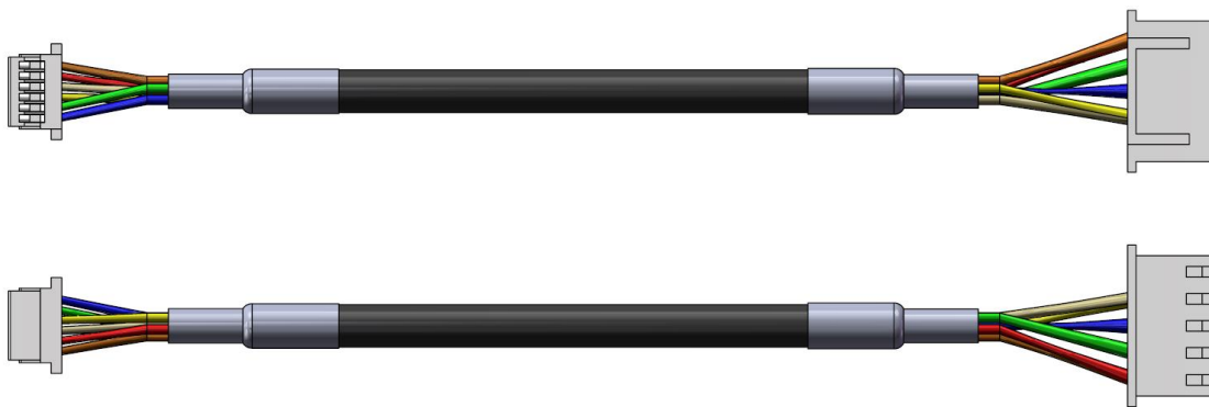
Figure 2-6 RPLIDAR S1 Interface Lead Schematic Diagram
