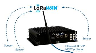
Cloud or on premise connection is based on standard IP Ethernet. The gateway automatically transforms LoRaWAN™ messages to a secure MQTT stream that is "pushed" on a remote MQTT server.
