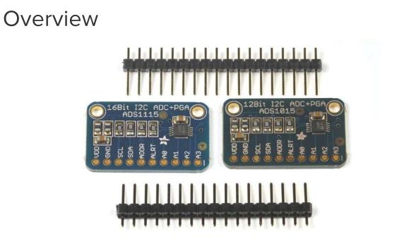
The ADS1115 and ADS1015 4-channel breakout boards are perfect for adding highresolution analog to digital conversion to any microprocessor-based project. These boards can run with power and logic signals between 2v to 5v, so they are compatible with all common 3.3v and 5v processors. As many of 4 of these boards can be controlled from the same 2-wire I2C bus, giving you up to 16 single-ended or 8 differential channels. A programmable gain amplifier provides up to x16 gain for small signals.
