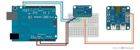
All input signals to these devices must be between ground potential and VCC. If your source signal produces negative voltages, they must be offset to fall within the GND to VCC range of the ASD1x15.
