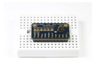
Position the breakout board Place the breakout board on the header pins.
