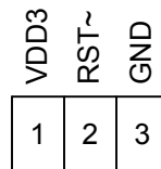
Figure 20. Host Power and I/O Header Connector
