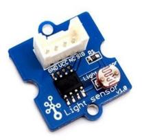
The light sensor, also known as the light dependent resistor (LDR). Typically, the resistance of the
