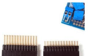
Next we will attach the header, there is a standard 'extra tall' header included in the kit. However, if you want to attach a cobbler or GertBoard, etc to the plate, you may want to opt for one of our stacking headers, they're extra long so you can plug in an IDC cable on top!
