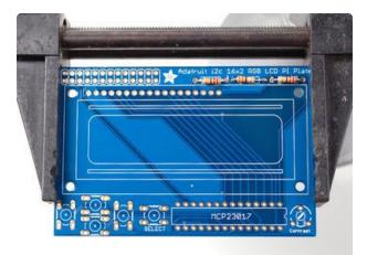
The two 220 ohm resistors RED and BLUE - named because they are the backlight series resistors for the RGB backlights on the LCDs. These resistors are colored Red Red Brown Gold.
