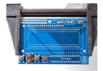
Next up we will place the buttons. These buttons are useful to send a signal to the Pi (say if you have a basic menu system). We have a 4-way 'direction pad' for up/down/left/right input and a button to the right called SELECT. These 5 buttons should be able to make 'talking' back to your project easy. These are connected to the I2C port expander chip so they require no extra pins on the Pi, our library does the work of reading whether they are pressed.
