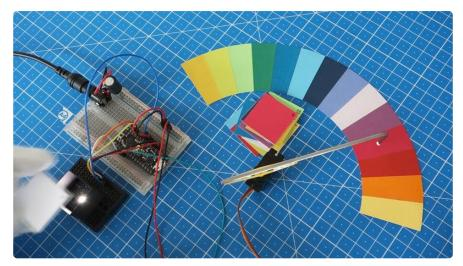
Identifying specific colors with a color sensor is not as simple as pointing the sensor at a color patch and taking a reading. There are many factors such as distance, field of view and ambient lighting conditions that can affect readings. Adafruit forum member systembolaget has developed a system capable of quickly and reliably identifying many different colors and has put together an excellent tutorial on the subject.
