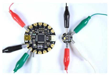
Both color sensors come with all surface mount components pre-soldered. The breakout-board version comes with an optional header for breadboard use. Soldering the header is a simple process:
