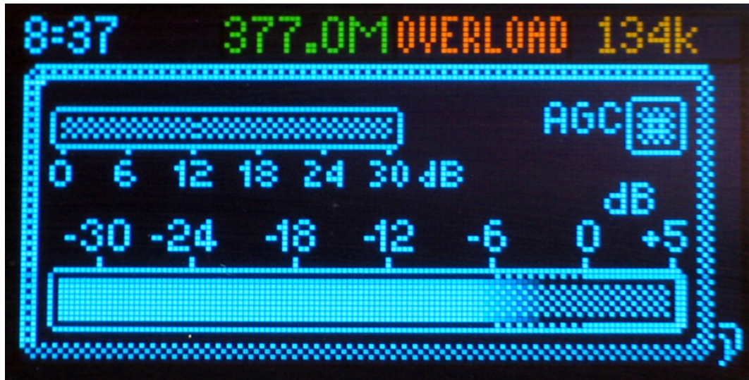
Figure 3: Real record display with monochrome VU meter.
