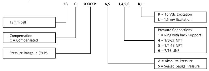
For example: **Part #13C3000PS4K** = 13 mm Cell, Compensated, 3000 psi, Sealed Gauge, 1/8NPT Port with 10 Vdc excitation.
