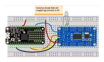
Board GND/ground to driver GND Board USB/5V to driver V+ and RGB LED anode (longest leg).
