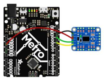
Connect VCC and V+ together to 3.3V (if a 4V+ power source is not available)
