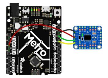
Keep VCC disconnected, and connect V+ to 4-17V
