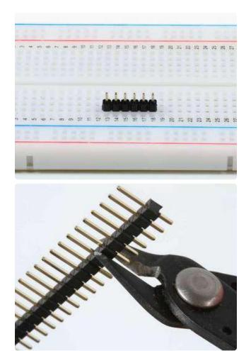
Position the header Cut to size first if necessary
