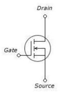
Internally, the "Source" of the FET is connected to Ground. But the Drain is left open. When switched on, the FET provides a path for current to flow from the output pin to ground.
