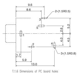
Tolerance: ±0.05(Printed—top view)
