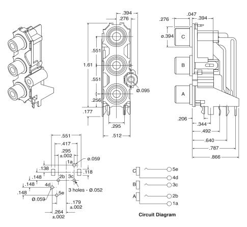
PCB Hole Layout ( Bottom View)
