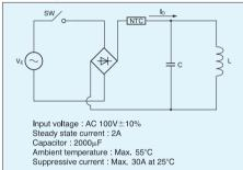
A suitable power thermistor for the above circuit is required to fulfill the following terms and conditions.
