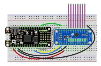
Board 3V to sensor VIN Board GND to sensor GND Board GND to sensor AD Board SCK to sensor SCK Board MOSI to sensor MOSI Board MISO to sensor MISO Board D5 to sensor CS (or use any other free digital I/O pin)
