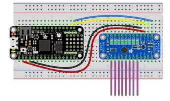
Board 3V to sensor VIN Board GND to sensor GND Board SCK to sensor SCK Board SDA to sensor SDA
