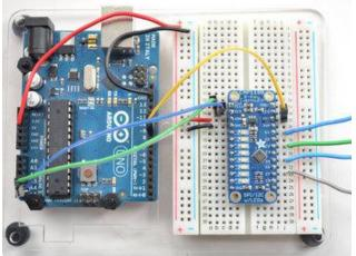
The reset pin is not required for use, but if you can spare a pin, it will make the system a little more rugged - the Arduino will do a hard reset of the CAP1188 on startup, connect RST to any digital I/O pin. In the library example code you can set up that pin in the CAP1188 object creation.
