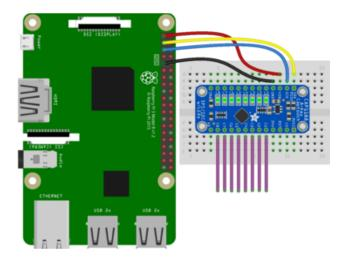
Pi 3V3 to sensor VIN Pi GND to sensor GND Pi SCL to sensor SCK Pi SDA to sensor SDA
