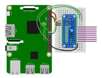
Pi 3V3 to sensor VIN Pi GND to sensor GND Pi GND to sensor AD Pi MOSI to sensor MOSI Pi MISO to sensor MISO Pi SCLK to sensor SCK Pi GPIO5 to sensor CS (or use any other free GPIO pin)
