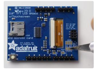
First start by taking a sharp knife and cutting the traces that connect to pins 11-13.
