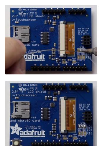
Next, apply a little solder to create a solder bridge on all three of the ICSP pads.
