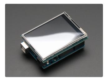
Plug the shield into your Arduino or Megashaped board. The GPIO pins are keyed and should only plug in one way.
