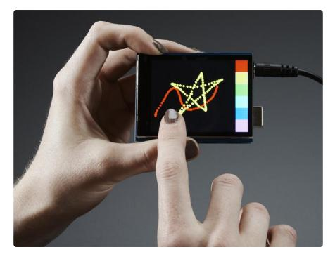
This shield uses the SPI port for sending data to the ILI9341 chipset display, and I2C for reading the TSC2007 resistive touch screen driver. That makes it work great with just about any board that is 'Arduino or Mega shaped' as long as they have the I2C SDA and SCL pins after pin D13, and the SPI 2x3 port. If you want to access the remaining pins, we recommend a WingShield ().
