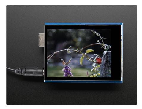
This display shield has a controller built into it with RAM buffering, so that almost no work is done by the microcontroller. This shield needs only a few pins: five SPI pins for the display (SPI + DC and CS), I2C and IRQ pin for the touch screen, and an optional backlight pin. One more pin can be used for the micro SD card if you want to read images off of it.
