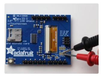
Next, take a multimeter set to the continuity setting and test that the traces were successfully separated.
