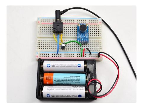
Connect the amplifier, battery pack and headphone jack as shown above.
