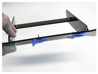
As with the main bezel, a little tape over the heads of these screws helps keep them in place.
