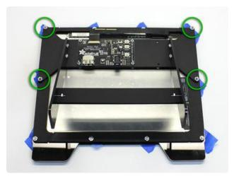
Carefully turn the stand over and lower it onto the four 5/8" screws. Add a nut to each and finger tighten.
