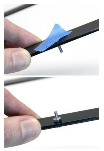
Insert a screw into each hole (1/2" or 5/8", as appropriate to the above diagram). The bezel will need to be flipped over later, so as you place each screw, secure it with a bit of tape, or you can use the nuts temporarily to keep the screws from sliding out (you'll need to remove these nuts later).
