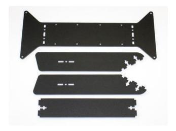
Locate these four laser-cut parts. For the sake of later explanation, let's refer to these (top-to-bottom) as the "bow tie," "legs" and "cross brace."
