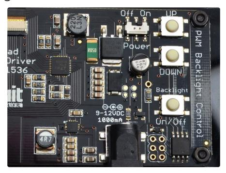
To control the backlight of the display, we use the awesome LT3754 LED driver from Linear Tech (). The great thing about this driver is it is a cross between an efficient boost convert and a fully-matched constant-current LED driver. The boost converter half can take 9-12VDC and boost it up to ~22VDC and the LED driver half makes sure that each LED strand is driven with exactly 18.5mA for perfectly distributed light (which gives better color representation).
