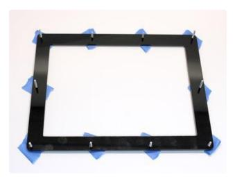
Once all the screws are placed, set the bezel face down on your work surface. Turn it so the "top" (with the longer screws) is at the...well...top.
