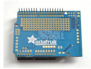
Start by sliding the 10 pin, 2 x 8 pin and 6pin stacking headers into the outer rows of the shield from the top. Then flip the board over so its resting on the four headers. Pull on the legs if necessary to straighten them out.
