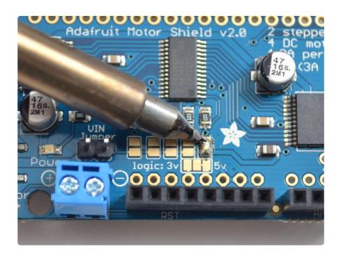
Board 0: Address = 0x60 Offset = binary 0000 (no jumpers required) Board 1: Address = 0x61 Offset = binary 0001 (bridge A0 as in the photo above)
