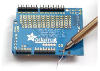
Solder in the two pins of the external power terminal-block
