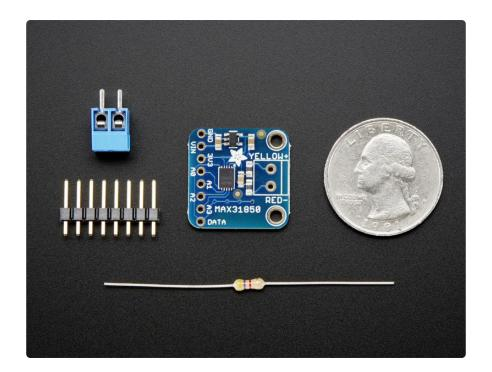
Comes with a 2 pin terminal block (for connecting to the thermocouple), 4.7K data line pullup resistor, and pin header (to plug into any breadboard or perfboard). Goes great with our 1m K-type thermocouple (http://adafru.it/270). Not for use with any other kind of thermocouple, K type only!
