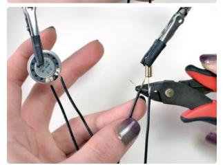
Hold a wire up to the speaker's pad and reheat the solder with your soldering iron. Hold it to the joint until the solder flows around the wire, then remove heat and hold the wire until the solder solidifies.
