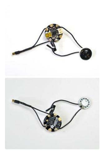
Your circuit is complete! Look it over, comparing it to the circuit diagram and double checking your solder joints.
