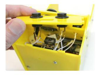
Friendly reminder: this is your last chance to add a USB mini WiFi adapter if you want! Plug it into the top USB slot. Leave the bottom slot open for a keyboard.
