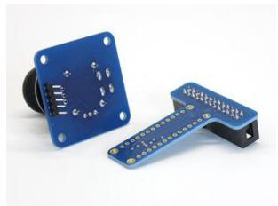
Make sure all your solder connections are smooth and clean, like tiny Hershey's Kisses®. There should be no solder balls or bridges, no gaps between pins and their corresponding pads.
