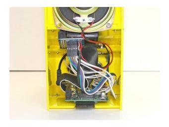
Stuff the wires into the back of the case, being careful not to dislodge the Cupcade board.
