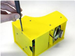
To install the back piece, you'll need to loosen <u>two</u> screws: the bottom and rearmost positions.
