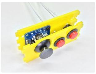
The quick-connect wires for the "A" and "B" buttons pass through corresponding cut-outs in the joystick support piece.
