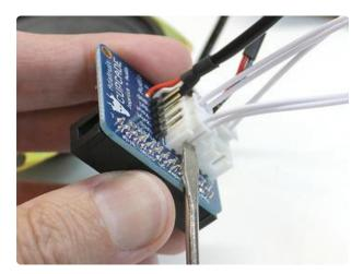
A small screwdriver is sometimes helpful when unplugging the buttons from the JST sockets. A little twist is usually sufficient...use common sense and be gentle.
