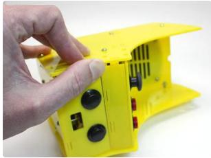
Install this fascia piece in a similar manner, then tighten the side screw back as it was.
