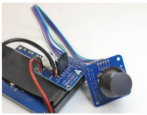
Connect the female jumper wires between the analog thumb joystick and the Cupcade board, making sure the same pins are connected at each end (e.g. GND to GND and so forth). Wire colors vary from batch to batch; yours might not match this photo, that's OK.
