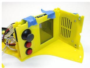
Fit the joystick and button supports into their own slots as you're working on this section. Use masking tape to hold these four pieces in alignment.
