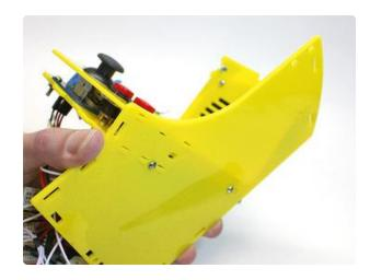
The trick now is to pick the whole thing up and feed these two screws through their corresponding holes in the side.
