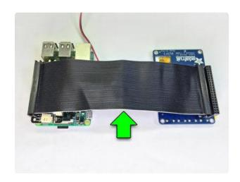
Disconnect the PiTFT from the Raspberry Pi, then plug the Arcade Bonnet in its place.
