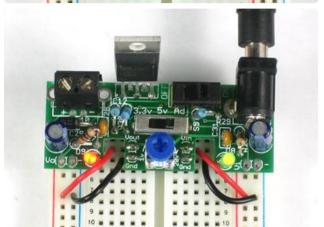
If your breadboard has nonstandard spacing, you can still plug it in using the header-breakouts in the middle.
