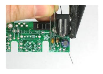
We will finish up the 'high voltage' power supply side by placing the green indicator LED. This LED will let us know that power is working! LEDs are diodes so they are polarized. If not placed correctly they will not work! So make sure you get this right.
