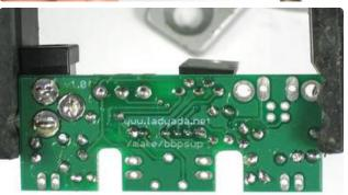
Finish off the 'low voltage' side by inserting the second 1.0K resistor R2 and the second 0.1uF ceramic capacitor C4.
