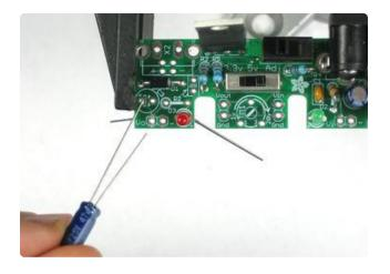
Next is the large electrolytic capacitor. Just like the other one, its polarized. Make sure the long lead goes into the (+) marked pad.
