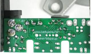
Solder and clip the three resistors.
