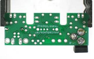
Now use yoru diagonal cutters to clip the long leads just above the solder joint.
