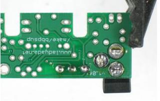
Tape or hold the switch in place while you solder all three pins.
