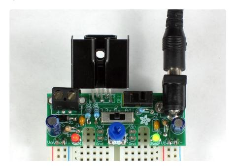
This project details the design of a very low dropout adjustable power supply. A good power supply is essential to electronic projects. While there are many existing designs for adjustable power supplies, this one makes improvements that make it more useful for hobby designs.
