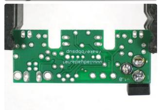
Flip over the PCB - you can either tape the DC jack down or use a finger to keep it place.
