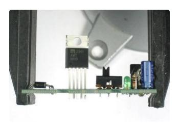
Now we will solder in the heart of the kit, the MIC2941 adjustable voltage regulator. The regulator must be placed correctly to work. Make sure that the big silver tab is at the edge of the PCB (theres a thick white line on the silkscreen to indicate it).
