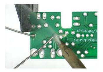
Now solder both wires to the PCB.
