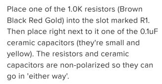
The resistor sets the brightness of the 'high voltage' indicator LED. The 0.1uF capacitor provides high frequency filtration to make the power supply cleaner.
