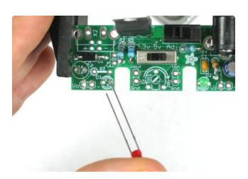
Now we will put in the capacitors and LEDs for the left hand "low voltage" side.
