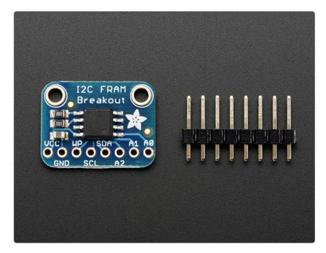
This particular FRAM chip has 256 Kbits (32 KBytes) of storage, interfaces using I2C, and can run at up to 1MHz I2C rates. Each byte can be read and written
