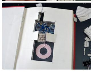
Don't forget to cut a channel for the USB cable!
