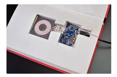
Make sure the book can close fully, and plug in the USB cable to verify the phone will charge when placed on top.
