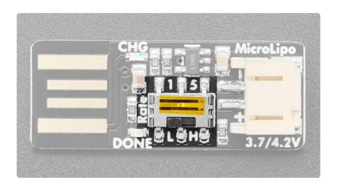
On the MicroLipo v2, there is a switch in the center of the board that replaces the jumper for changing between 100mA and 500mA charging modes. 100mA is labeled with 1 above the switch and L below the switch (for low mode). 500mA is labeled with 5 above the switch and H below the switch (for high mode).
