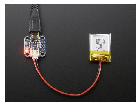
You can plug in either the battery first or the USB port first. We provide a JST jack since the large number of batteries we carry come with a JST PH connector or cable
