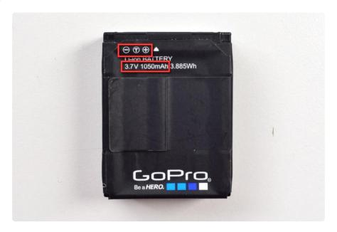
You can see its a 3.7V 1000mAh battery. That means we can charge it at 500mA max rate if we wish.
