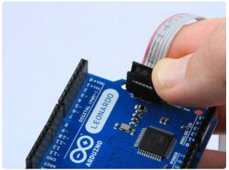
Attach the 6-pin end to the ICSP header on the Leonardo as shown. Make sure to align the edge with the red-stripe so that it is closest to the "LEONARDO" logo on the board.
