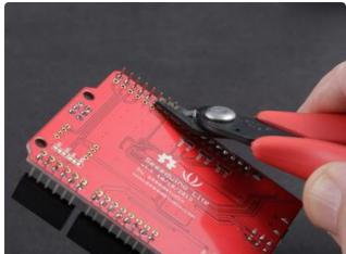
Trim the pins on the back and you are ready for the final assembly of your Pixy Pet!
