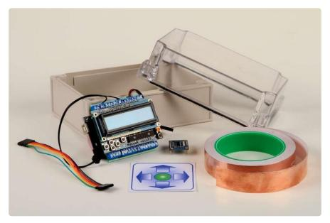
Capacitive touch sensors are a great way to add external controls to a waterproof enclosure. There is no need to drill holes or worry about gaskets and O-rings. These sensors will detect your touch right through the plastic case!
