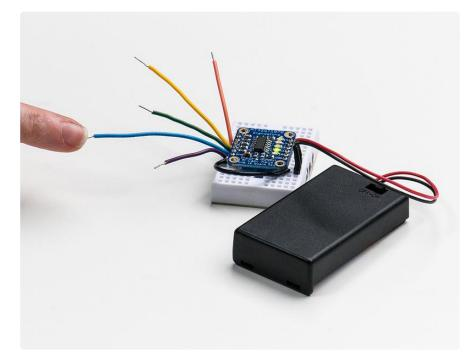
The 5-pin momentary breakout can be powered with anything from 1.8V to 5.5VDC. Just connect ground to GND and the positive voltage to VDD. This sensor does not
