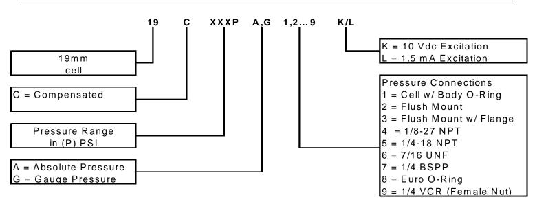
For example: Part **#19C100PA4K** = 19 mm Cell, Compensated, 100 psi, Absolute, 1/8NPT Port, with 10 Vdc excitation.
