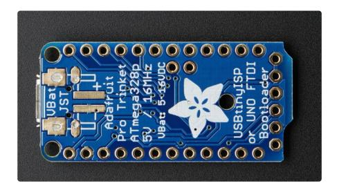
On the bottom there's a spot for a <u>2-pin JST-PH connector</u> (http://adafru.it/1769). this is optional and can be soldered on by hand. It will let you use a lipoly or <u>AAA battery pack</u> (http://adafru.it/727) or <u>a JST cable</u> (https://adafru.it/drM) for other power input. It's connected to the GND and VBAT pins
