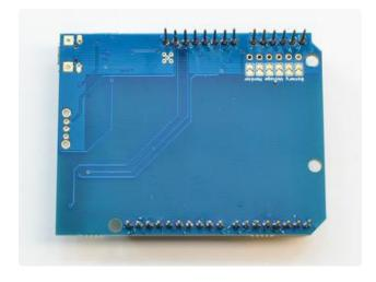
Check your work, especially the power (5V) and GND pads! Make sure there's no bridged solder connections
