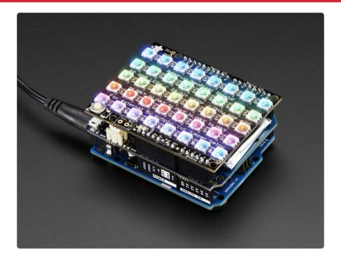
The onboard boost converter can provide at least 500mA current, and can peak at 1A. There's an onboard fuse to protect against higher current draws which could damage
