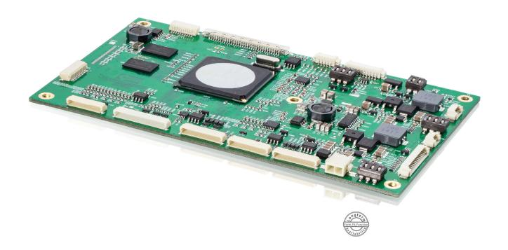
Low-Profile Full-HD-Flatpanel Controller with SD/HD-TV Video-Decoder
