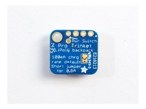
For use with Adafruit LiPoly/Lilon batteries only! Other batteries may have different voltage, chemistry, polarity or pinout.
