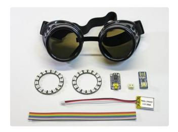
The kit version includes our costume goggles (), two NeoPixel rings (), a Trinket M0 () or Trinket Mini Microcontroller (), JST connector (http://adafru.it/1769), rechargeable 150 mAh LiPoly battery (), enough wire for all the connections, plus a USB battery charger ().
