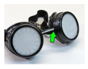
Screw the lenses in place, being super extra careful not to gouge the wires!
