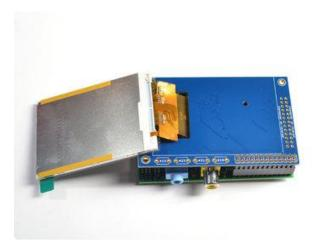
Place the PiTFT shield on top so all the pins stick through the connector on the side. Gently flip the TFT so its off to the side and wont be in your way while you solder
