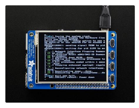
This design uses the hardware SPI pins (SCK, MOSI, MISO, CE0, CE1) as well as GPIO #25 and #24. All other GPIO are unused. Since we had a tiny bit of space, there's 4 spots for optional slim tactile switches wired to four GPIOs, that you can use if you want to make a basic user interface. For example, you can use one as a power on/off button.
