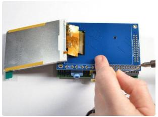
Heat up your soldering iron, and grab some solder. Start by tack-soldering one of the corners while pressing on the plate to make it sit flat. Once you have one or two pins done you can continue to solder each of the pins.
