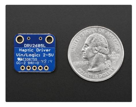
According to the product page, it can be used with both LRA (Linear Resonance Actuator) and ERM (Eccentric Rotating Mass) type motors <u>but we have only used it</u> with our little vibration pancake ERM. (https://adafru.it/dDc)
