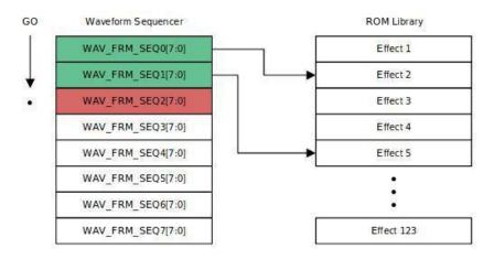
You access the Waveform Sequencer by using the sequence property and providing an index for the slot location. To specify the effect, use the special Effect class provided in the library, giving it the effect number. For example, here is how to load Effect ID No. 1 "Strong Click - 100%" into slot 0 of the sequence:
