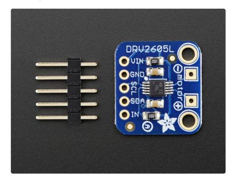
This chip is controlled over I2C - after initialization, a 'string' of multiple effects can be strung together in the chips memory and then triggered to actuate in a row. The built in effects are much much nicer than just 'on' and 'off' and will make your haptic project way nicer feeling.
