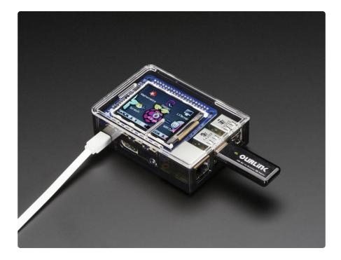
This design uses the hardware SPI pins (SCK, MOSI, MISO, CEO, CE1) as well as GPIO #25. All other GPIO are unused. Since we had a tiny bit of space, there's 4 flat tactile switches wired to four GPIOs, that you can use if you want to make a basic user interface. For example, you can use one as a power on/off button.
