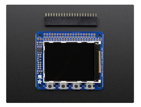
Comes as a fully assembled display PCB and an additional 2x20 GPIO header. Some light soldering is required to attach the 2x20 GPIO header to the HAT but it's fast and easy for anyone with a soldering iron and solder
