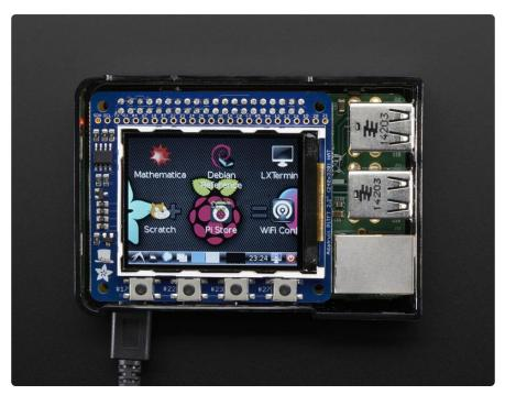
The cute PiTFT got even more adorable with this little primary display for Raspberry Pi in HAT form! It features a 2.2" display with 320x240 16-bit color pixels. The HAT uses the high speed SPI interface on the Pi and can use the mini display as a console, X window port, displaying images or video etc. Best of all it plugs right in on top of your Model A+ or B+ and fits into our case quite nicely.
