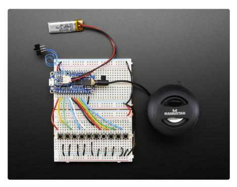
You can see each button connects to the trigger pin, and then the other side to ground. For this demo I'm using the Lipoly backpack but you can power any other way. When buttons are pressed, the audio files on the board get triggered!
