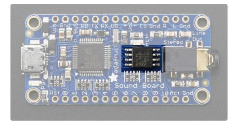
This is the onboard flash chip. It's basically like a little SD card, but soldered directly onto the PCB. These chips can store a few megabytes. This doesn't seem like much but for most audio effects, you don't need hours of music. You can store a couple minute's worth of compressed OGG on a 2M flash chip.
