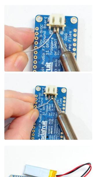
Solder all four pads - two mechanicals on the side, and two power coming out the end.
