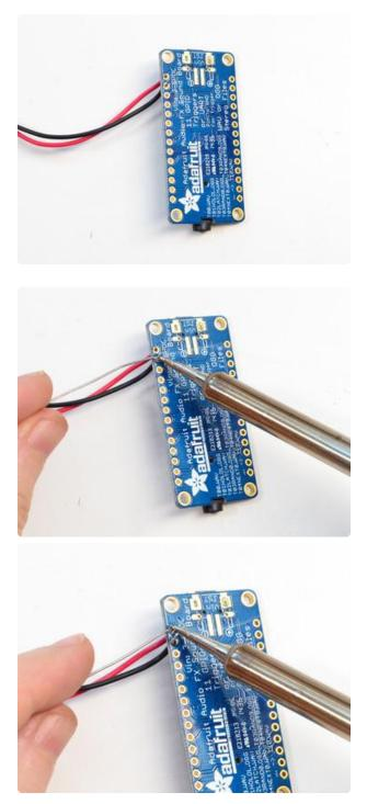
For most battery packs the red wire is the positive wire, connect that to Vin. The black wire is ground, connect that to GND.
