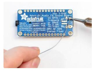
Start by melting some solder onto one of the side pads of the JST footprint on the bottom
