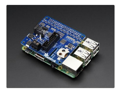
Works with any of our 16x32, 32x32 or 32x64 RGB LED Matrices with HUB75 connections (https://adafru.it/emd). The latest "Rev C" HAT also supports 64x64 matrices by soldering a small jumper on the PCB. You can even chain multiple matrices together for a longer display - we've only tested up to 32x128 but it works just fine. The bigger the display the harder it is on the Pi, so keep that in mind if you're using a lower-powered Pi Zero.
