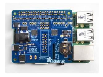
Place the HAT on top so that the short pins of the 2x20 header line up with the pads on the HAT
