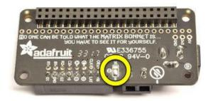
If you're using a 64x64 RGB matrix and either a Bonnet or a Rev C HAT, use your soldering iron to melt a blob of solder on the bottom solder jumper so the middle pad is 'shorted' to 8. (This is compatible with 64x64 matrices in the Adafruit store. For 64x64 matrices from other sources, you might need to use 16 instead, check the datasheet.)
