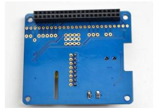
Check your work! Make sure all the solder points are clean and not shorted or cracked or dull
