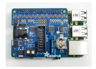
Shut down your Pi and remove power. Plug the HAT or Bonnet on so all the 2x20 pins go into the GPIO header.
