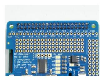
Check over your work so far, make sure each solder point is shiny, and isn't bridged or dull or cracked
