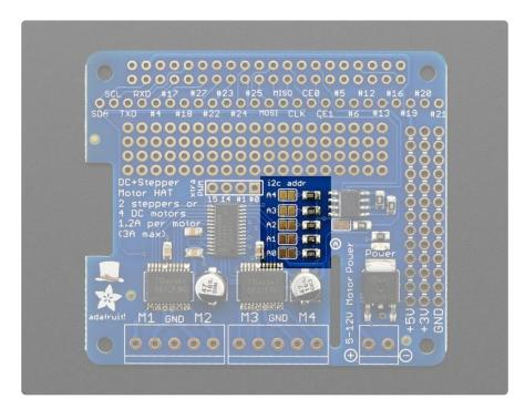
Board 0: Address = 0x60 Offset = binary 0000 (no jumpers required) Board 1: Address = 0x61 Offset = binary 0001 (bridge A0) Board 2: Address = 0x62 Offset = binary 0010 (bridge A1, the one above A0) Board 3: Address = 0x63 Offset = binary 0011 (bridge A0 & A1, two bottom jumpers) Board 4: Address = 0x64 Offset = binary 0100 (bridge A2, middle jumper)
