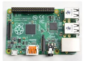
Start by plugging the 2x20 header into a Raspberry Pi, this will keep the header stable while you solder. Make sure the Pi is powered down!
