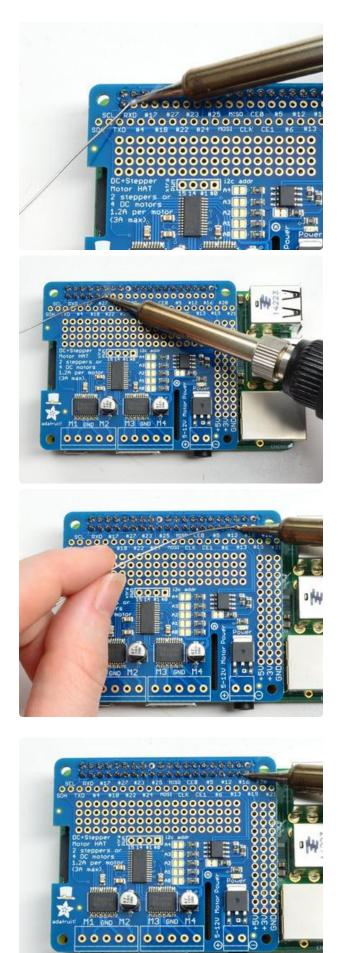
Flip the board around and solder all the connections for the other half of the 2x20 header
