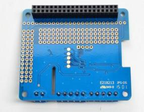
Flip over the board and solder in all of the terminal block pins
