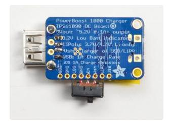
Flip over to solder the three pads in place
