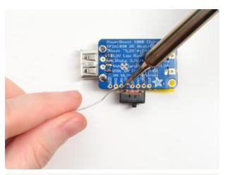
Solder in all three pins with any kind of solder making sure you have a good connection
