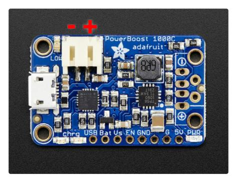
The USB connector can be soldered on to create a portable 'USB power pack'. The two data lines on USB have resistor dividers that match Apple charger values for 1A charge rate so that you can plug any iOS device in to charge. 99% of other phones, devices and tables are totally cool with these resistors as well. You can always short the D+ and D- lines if you happen to have a phone that wants shorted data lines.
