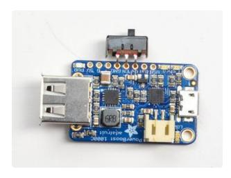
The switch will go into the breakout header, and attach to VS EN and GND The switch is symmetric so as long as those three pins are attached to the switch you are good to go
