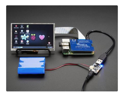
The PowerBoost 1000C has at the heart a <u>TPS61090 boost converter from TI</u> (https://adafru.it/duQ). This boost converter chip has some really nice extras such as low battery detection, 2A internal switch, synchronous conversion, excellent efficiency, and 700KHz high-frequency operation. Check out these specs!
