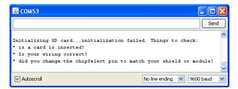
It couldn't even initialize the SD card. This can also happen if there's a soldering or wiring error or if the card is really damaged.
