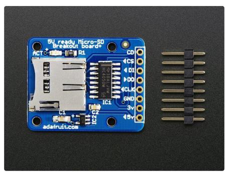
If you have a project with any audio, video, graphics, data logging, etc in it, you'll find that having a removable storage option is essential. Most microcontrollers have extremely limited built-in storage. For example, even the Arduino Mega chip (the Atmega2560) has a mere 4Kbytes of EEPROM storage. There's more flash (256K) but you can't write to it as easily and you have to be careful if you want to store information in flash that you don't overwrite the program itself!
